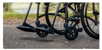
Adjustable and detachable leg rests designed for ease of storage and transport
